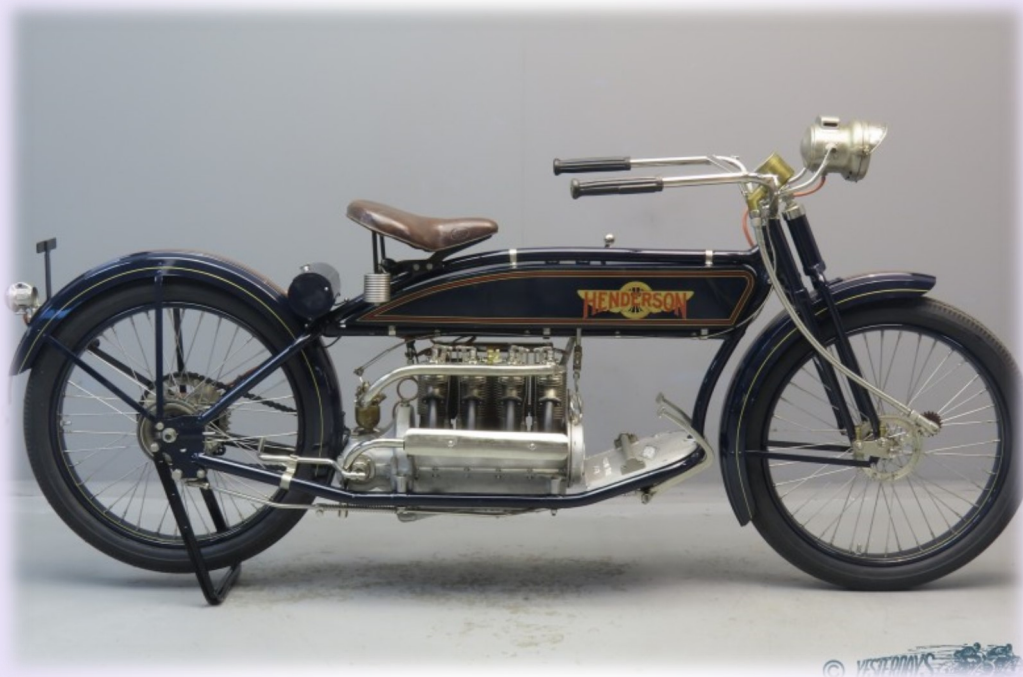
Henderson 1914 "Model C" 1065 cc I.O.E. four cylinder engine
